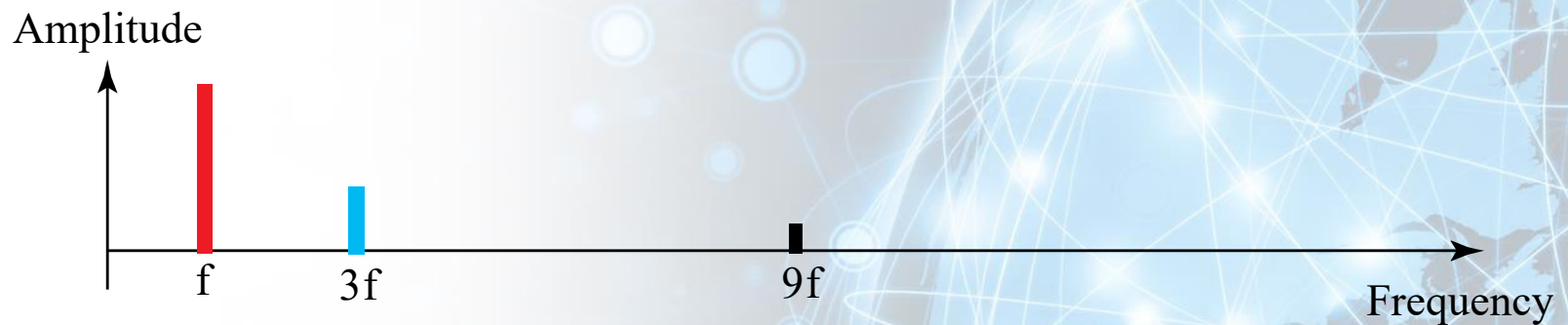
b. Frequency-domain decomposition of the composite signal
