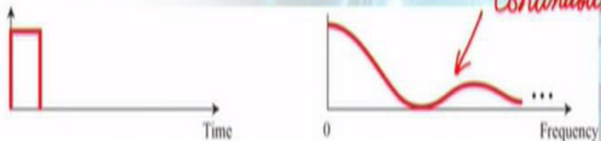
b. Time and frequency domains of nonperiodic digital signal
